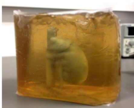
Fig. 4. Human-kidney phantom immersed in a background water-based gel.
